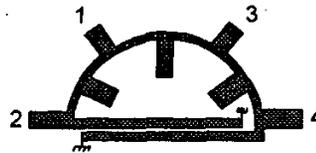
Fig.7 Layout of a compact coupler based on the coupled line short circuited at its diagonal
