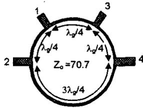
Fig.1 Layout of the conventional ring Coupler based on  $\lambda/4$  line
