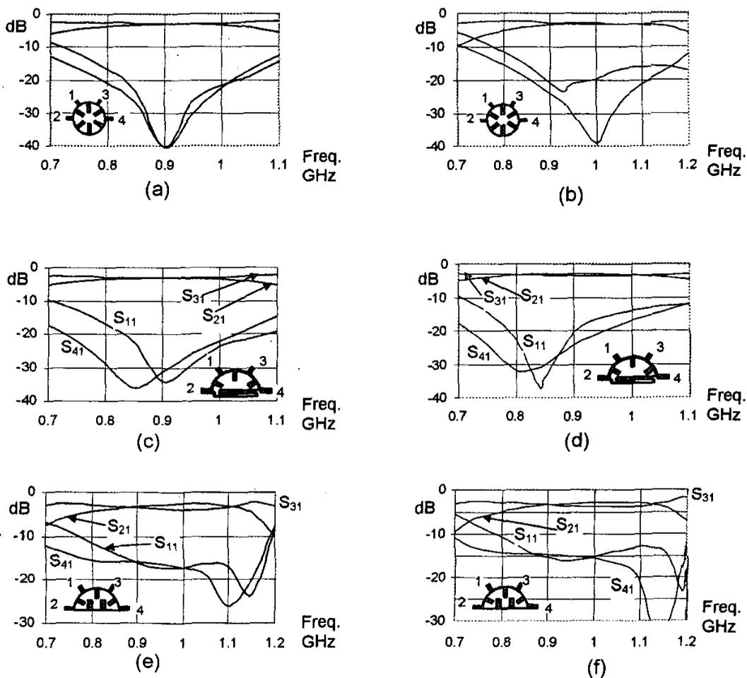
Fig.9 simulation and measured results of 3-dB ring coupler designed at 900MHz
