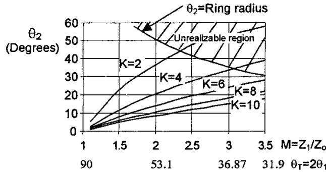
Fig.3 Design curves for the circuit in Fig. (2b) to be equivalent to  $\lambda/4$  line in Fig. (2a)
