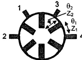
Fig.4 Ring coupler layout based on T-shape circuit equivalent in Fig. 1
