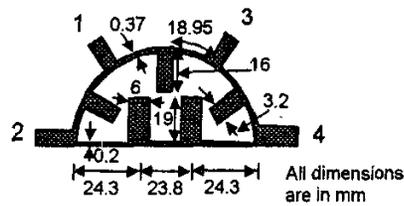
Fig.6 Layout of a compact coupler based on the T- shape circuit in Fig.2(b) and the  $\Pi$  circuit equivalent in Fig.5(b)
