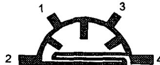
Fig.8 Layout of a compact coupler, the three quarter wavelength line formed in serpentine shape
